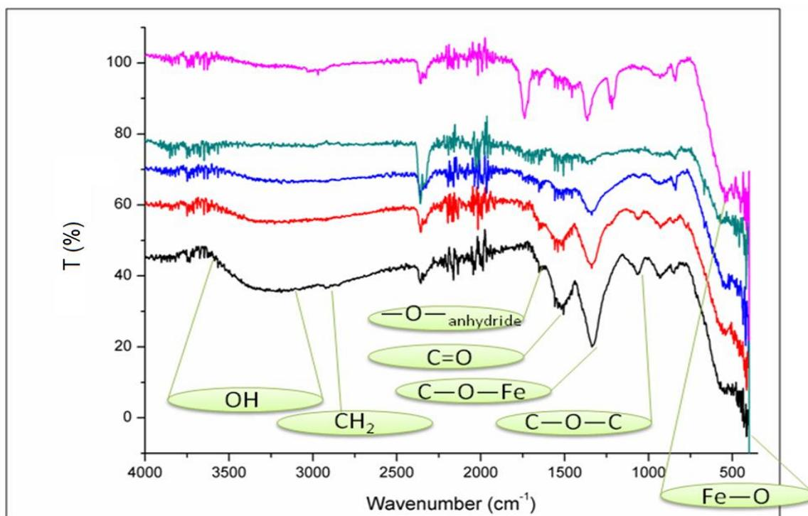
Figure 5. FTIR spectra of iron oxide nanoparticles surface modified using Tween-80.
