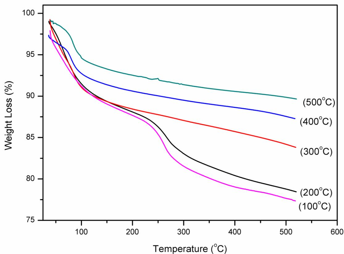
Figure 6 TG curves of the iron oxide nanoparticles annealed at different temperatures
