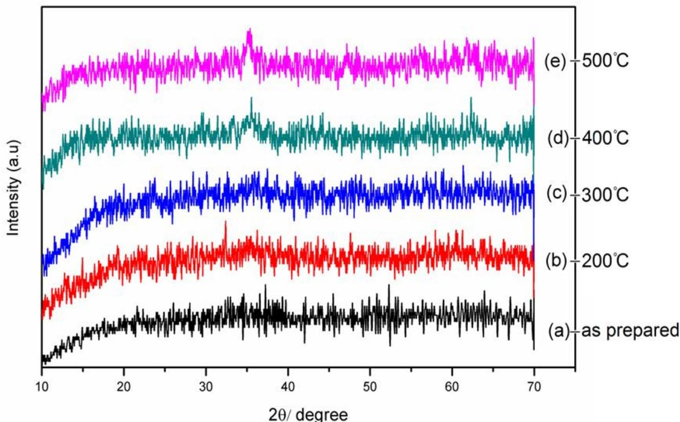
Figure 2 PXRD patterns of iron oxide nanoparticles prepared at (a) 90 °C and annealed at (b) 200 °C (c) 300 °C (d) 400 °C (e) 500 °C.
