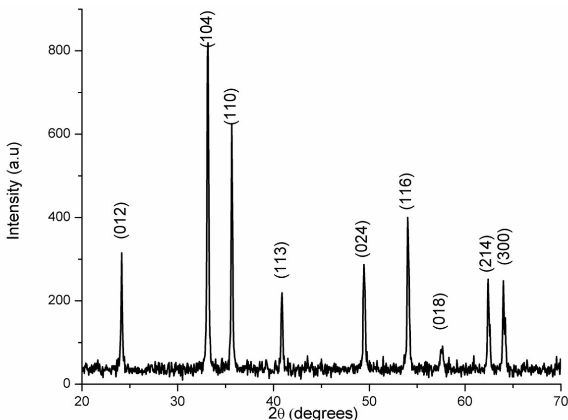
Figure 3 PXRD patterns of iron oxide nanoparticles prepared at 90 °C and annealed at 400 °C for 2 hours.
