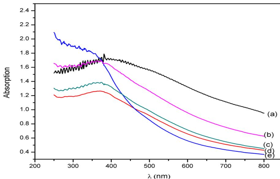
Figure 1. UV/Visible spectra of surface modified iron oxide nanoparticles
